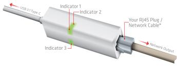
Indicator 1: this indicator turns Green to indicate connection establishment between host PC and Ethernet source.
